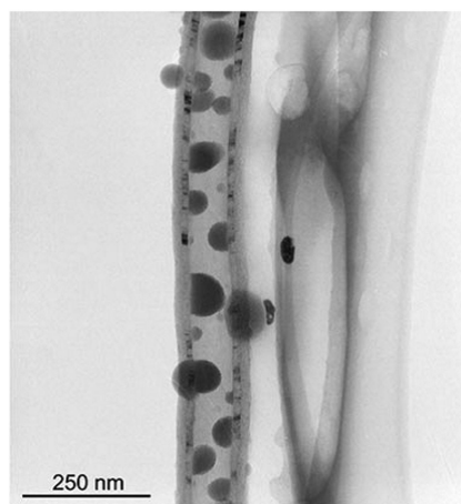
Figure 8. TEM micrograph showing a carbon nanofibers/LCP composite obtained by a non aqueous sol-gel route by Sarapulova et al. (74). Reprinted with permission from ref. (74). Copyright (2012) Springer publishing.
