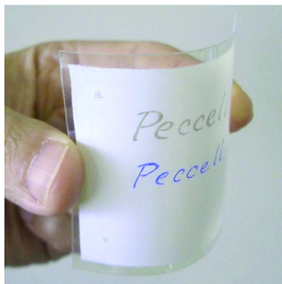
Figure 12. Image of a TiO 2 -coated ITO-PEN substrate for flexible DSC. (Reproduced with permission from reference (87). Copyright 2007 The Electrochemical Society.)
